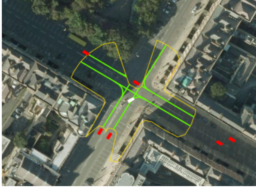
Fig. 4.9: Conversion of polygon to one-dimensional ranges
